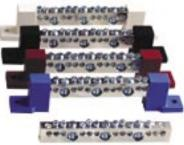
Use for adding more wire terminations or for isolating multiple positive / negative circuits. All TBB and GBB models have three #1/0 to 14 AWG and eight #6 to 14 AWG screw type compression terminals, which means no ring lugs required. Available with black, white and
